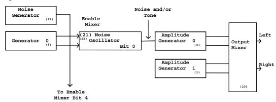
Using this mixer allows either noise or tone or both or nothing to be passed to a single amplitude register and so to a precise position in the stereo field.
